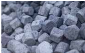
Silicon carbide to increase the silicon content in the iron
