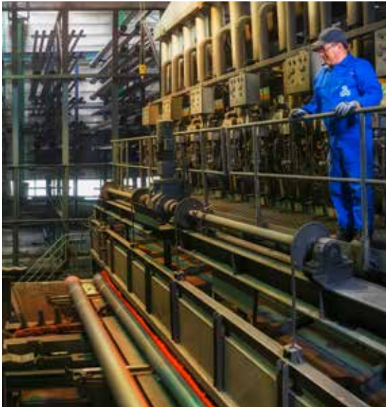
Annealing furnace to improve material properties
