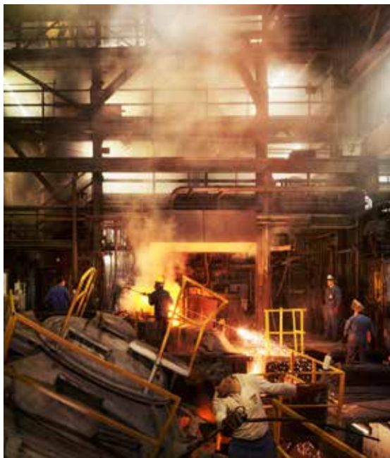
Cupola furnace with channel furnace in the foreground
