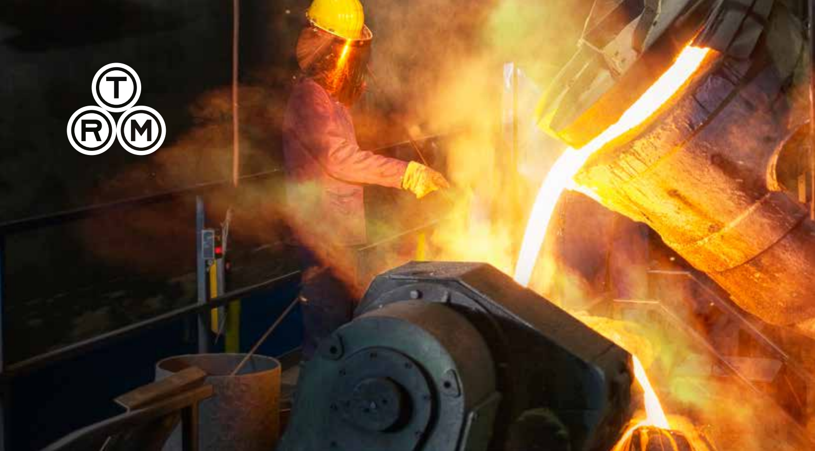
Filling the centrifugal casting machine
